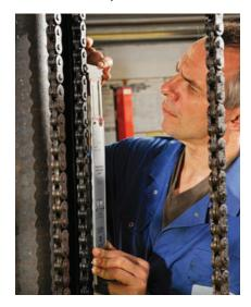
In the United States for example, Carolina Handling - part of the Raymond Truck Sales and Servicing Network - has recently equipped each of its 200 mobile forklift field service technicians with an FB chain wear gauge.
